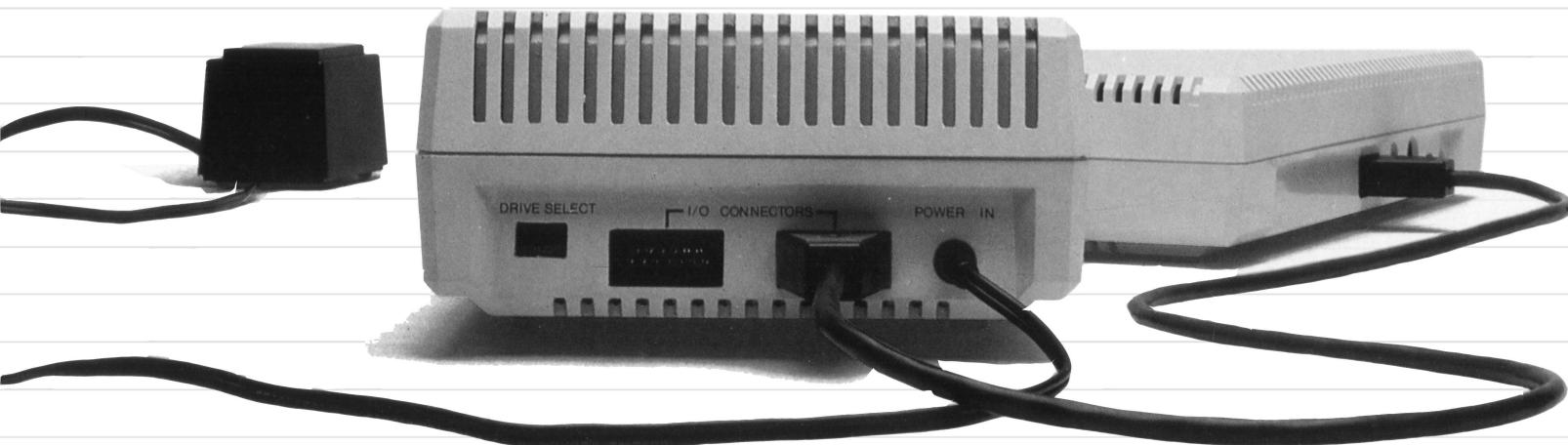
As many as four disk drives, in addition to other components, can be connected to the ATARI Home Computer by Serial I/O Cables supplied with components. To install multiple drives, connect a cable between one I/O CONNECTOR jack on the first drive and a PERIPHERAL jack on the computer console. Connect another cable between the remaining I/O CONNECTOR jack on the first drive and an I/O CONNECTOR jack on the second drive. Connect additional components in the same manner.
